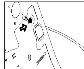
3. 拆下油门拉线
